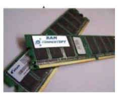
Dynamic RAM is more complicated to interface to and control and needs regular refresh cycles to prevent its contents being lost. However, DRAM uses only one transistor and a capacitor per bit, allowing it to reach much higher densities and, with more bits on a memory chip, be much cheaper per bit. SRAM is not worthwhile for desktop system memory, where DRAM dominates, but is used for their cache memories..
